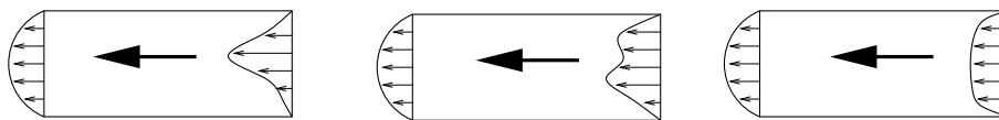
FIGURE 1.1. Most local variations in the boundary conditions are not “transmitted” through the component, and in a global, network view, despite the distributed nature, average or lumped variables can be selected.
